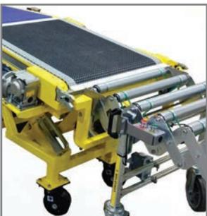
**Conveyor Integration:** Destuff-IT™ machines can be integrated with a variety of conveyor types, including flexible roller conveyor, telescopic belt conveyor and cascading belt conveyor.
