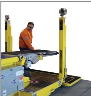
**Drive System and Operator Sensors:** Each Destuff-IT™ machine is easily moved from dock to dock under its own independent power. These self-propelled machines have an integrated DC drive and steering system capable of negotiating dock leveler slopes and transition plates.
