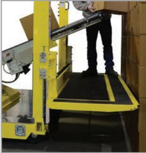
**Operator Platform:** The sturdy operator platform has a rubber ergo mat with treaded surface. In addition, the platform is able to reach a maximum vertical height of 26" (660 mm) which aids up to two workers in reaching the top of the box wall. Platforms are available in a standard width [22" (559 mm)] or an extended width [33" (838 mm)] and have a capacity of 550 lbs (250 kg).
