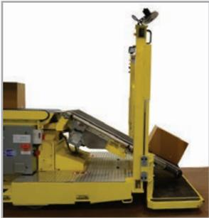
**Pivoting Conveyor:** The pivoting conveyor enables an operator to adjust the horizontal and vertical position of the belt for optimal positioning to the box wall. Workers use a handle located at the side of the conveyor to release a brake allowing manual rotation (side to side) of the conveyor. For tilting up and down, the operator simply twists the handle much the same as a motorcycle throttle. Specifications for the pivoting conveyor include:
