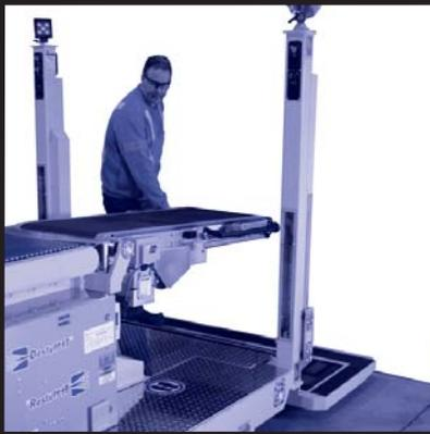
**DRIVE SYSTEM & OPERATOR SENSORS:** Each Destuff-IT™ machine is easily moved from dock to dock under its own independent power. These self-propelled machines have an integrated DC drive and steering system capable of negotiating dock leveler slopes and transition plates.
