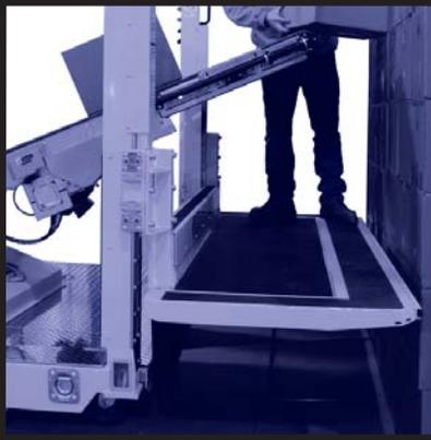
**OPERATOR PLATFORM:** The sturdy operator platform has a rubber ergo tread surface. In addition, the platform is able to reach a maximum vertical height of 26" (660 mm) which aids workers in reaching the top of the box wall. Platforms are available in a standard width [22" (559 mm)] or an extended width [33" (838 mm)] and have a capacity of 550 lbs (250 kg).
